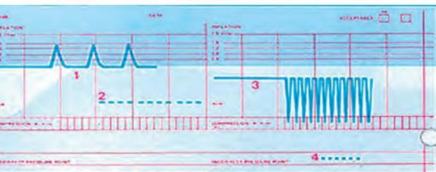
The Recording Resusci Anne provides feedback, printing out an accurate recording of ventilation and compression quality.
