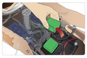
3 Snap the battery clamp back into place over the batteries.
