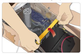
2 Insert both batteries into the battery tray.
