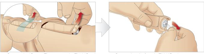
3 Remove the IO tape. Then remove the Tibial IO unit from the leg.
