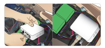
Open the pelvis and locate the router: Remove the two Ethernet cables and black power cable.
