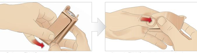
7 Fit the new Tibial IO pad into the chassis.
