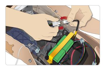
After connecting the batteries, connect the Patient Simulator to the external power supply (12V to 24V) while turned OFF.
