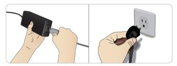
Plug the power supply into a wall outlet and connect the power cable to the power inlet on the Patient Simulator's power panel.
