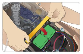
4 Connect the corresponding battery cables from the batteries to the torso.
