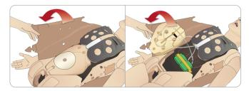
4 Open the Stomach Foam to one side, taking care not to tug on the connecting tubes and cables.
